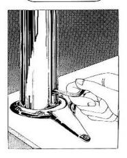
4) Using the provided allen wrench, tighten the expansion screw. This will secure the leg on the bracket. DO NOT over tighten the expanding screw or damage may result.
