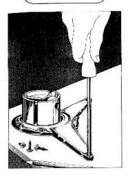
**2)** By using the mounting template provided with the table legs drill pilot holes. Attach mounting bracket using screws provided or your own.
