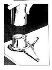
3) Slide table leg over the bracket so that expansion screw and square slot in table leg line up.
